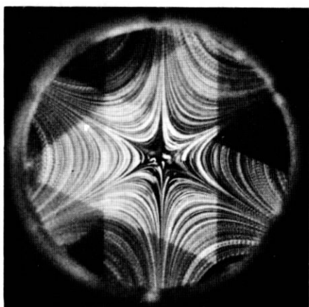
The six roll mill: experimental observations and computer simulations of the patterns illustrating elliptic umbilic critical point.
