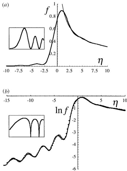
**Figure 2.** (a) Thick curve, fake caustic diffraction function (13); thin curve, geometrical-optics approximation (15); inset, genuine caustic (rainbow) diffraction function  $\text{Ai}^2(-\rho)$ . (b) Full curve, measured intensity from a scanned photograph of a fake caustic; dots,  $\ln f(\eta)$ , calculated from (13); inset,  $\ln\{\text{Ai}^2(-\rho)\}$ .
