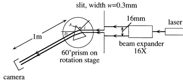
Figure 1. Experiment for observing a fake caustic.
