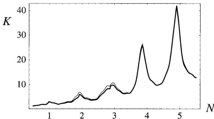
Figure 2. Petermann factor for the lowest-loss mode, for  $M = 1.5$ , computed exactly, by matrix diagonalization (—), and according to the asymptotic theory (---).
