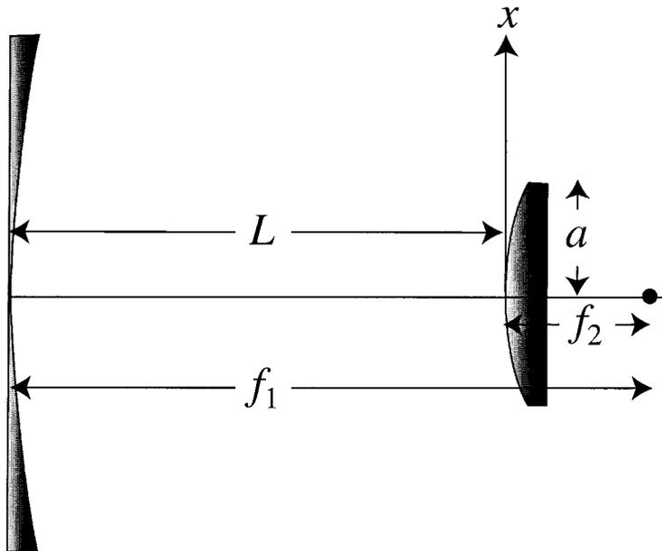
Figure 1. Strip resonator cavity corresponding to a confocal unstable laser.
