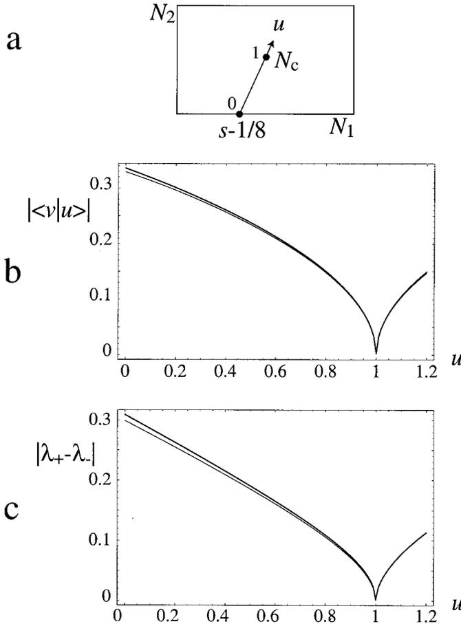
Figure 5. (a) Path in the complex  $N$  plane passing through a degeneracy  $N_c$ ; (b) corresponding behaviour of the self-overlap  $|\langle v|u \rangle|$ , calculated exactly (—) and with the asymptotic approximation (---), for  $M = 1.5$ ; (c) as (b), but for the eigenvalue difference  $|\lambda_+ - \lambda_-|$ .
