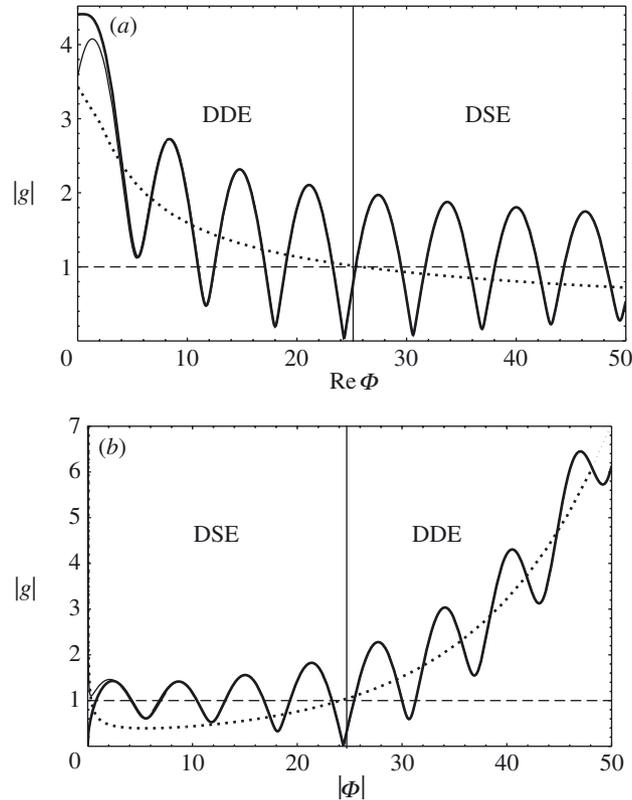
Figure 1. Modulus  $|g(\Phi)|$ , showing the transition between DSE and DDE for the Fresnel integral  $g_1(\Phi)$  (equation (3.4)) of § 3 *a*: (a) on a line with  $\text{Im } \Phi = 2.2$ ; (b) on a ray with  $\arg \Phi = \pi/35$ . Thick curves, exact  $|g|$ ; thin curves, the approximation (2.6); dashed lines, subdominant contribution (unity) to  $g$ ; dotted curves, dominant contribution to  $g$  (first term of (2.6)).
