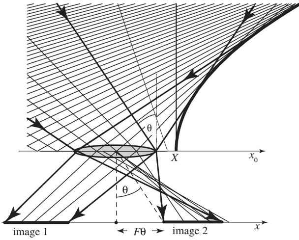
**Figure 2.** Formation of two images by rays focused onto a caustic curve. Each image is spread as illustrated in figure 3, and the rays shown in bold are those encountering the edges of the lens.
