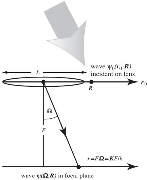
**Figure 1.** Notation for lens plane, in which the incident wave  $\psi_0$  can be shifted by  $\mathbf{R}$  relative to the lens of aperture  $L$  and focal length  $F$ , and the focal plane, where light coming from directions  $\Omega$  is imaged.
